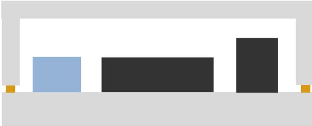
Figure 9: Heat conductor traces between LCP substrate and LCP frame or lid
