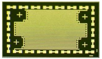
Figure 10: Test chip used for soak tests
