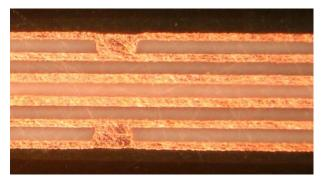
Figure 1. Ultra-thin 6-layer multilayer stackup with 25  $\mu$ m thick LCP layers. Minimum via diameter: 30  $\mu$ m. Total thickness: 182  $\mu$ m.
