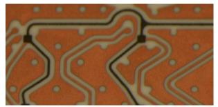
Figure 4. Cu-Constantan (black traces) thermocouples (50  $\mu$ m x 50  $\mu$ m) on a LCP substrate. The structure will be covered with another layer of substrate material and can be formed into any desired shape.
