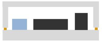
*Figure 9: Heat conductor traces between LCP substrate and LCP frame or lid*
