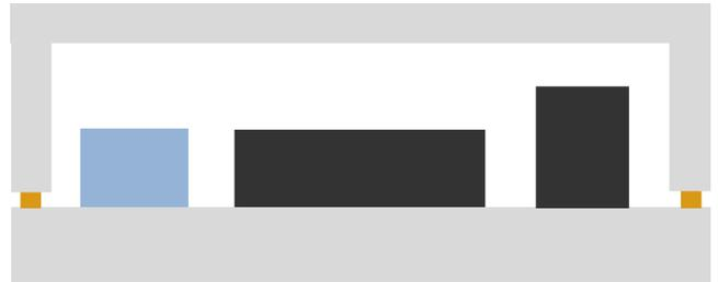
Figure 9: Heat conductor traces between LCP substrate and LCP frame or lid
