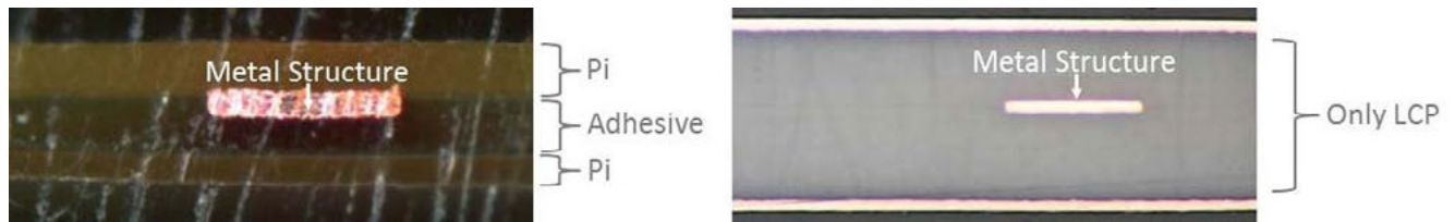
Figure 3: Assembling of different Pi layer made by adhesives (left); several LCP layer thermally bonded (right).
